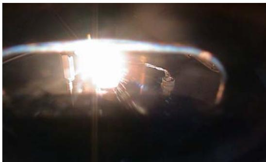
Figure 8. TVA plasma running in beryllium vapours.(At Nuclear Fuel Factory in Pitesti facilities)
