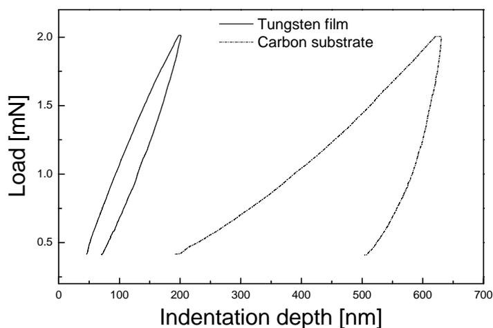
Figure 5. Comparison of loading / unloading curves for W and substrate at maximum indentation load of 2 mN.
