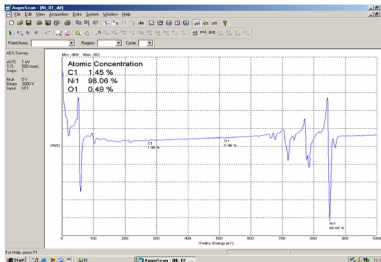
Figure 7. The results of measurements of C and O concentrations in Ni coatings of 2.5  $\mu$ m using Auger electron spectroscopy (AES) techniques. Values of 1.45%C, 0.49%O have been obtained.
