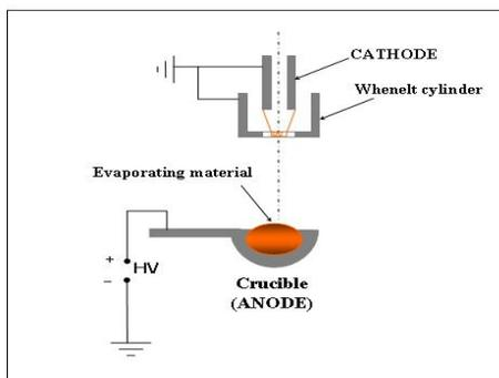
*Figure 1. TVA principle scheme.*
