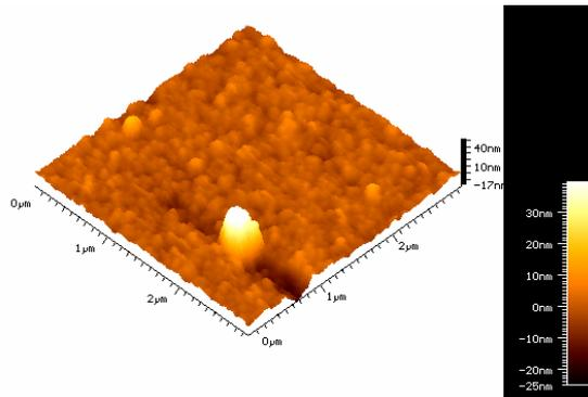
Figure 6. AFM image of the W film obtained by an atomic force microscope in contact mode atomic force microscope.
