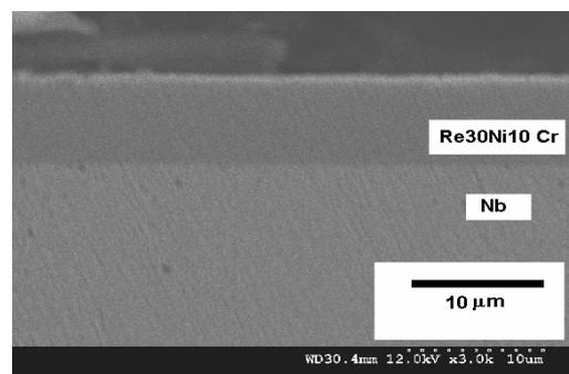
*Figure 2. Cross sectional view of the Re30Ni10Cr film.*
