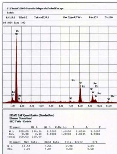
Figure 4. Typical spectrum of EDX analysis of W coating.
