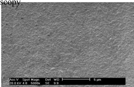
Figure 10. SEM image of the Be film deposited on stainless steel by thermionic vacuum arc (TVA) method
