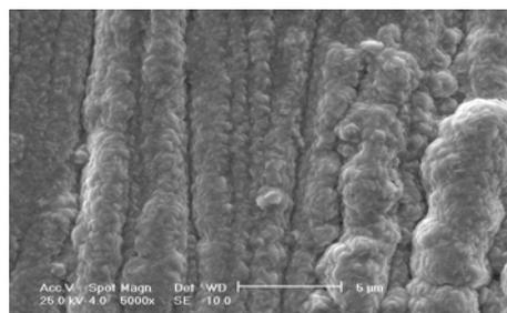
*Figure 3. SEM image of W film on metal substrate*
